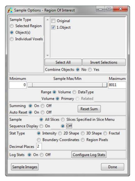
20. Click Sample Images to run the measurement algorithm. The ROI Stat Log window will be returned. Click the Save button to save out the data as a .stats file, which can be imported into a spreadsheet for further analysis.
