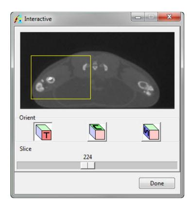
Open the cropped data set in the Oblique Sections module (Display > Oblique Sections). Open the Orthogonals tool (Tools > Orthogonals). Right-click in the coronal view and double the size of the display. Use the slice slider to navigate through the coronal slices.
