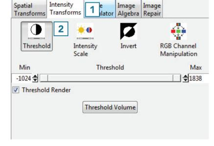
**Threshold slider:** The Threshold double-ended slider bar allows users
